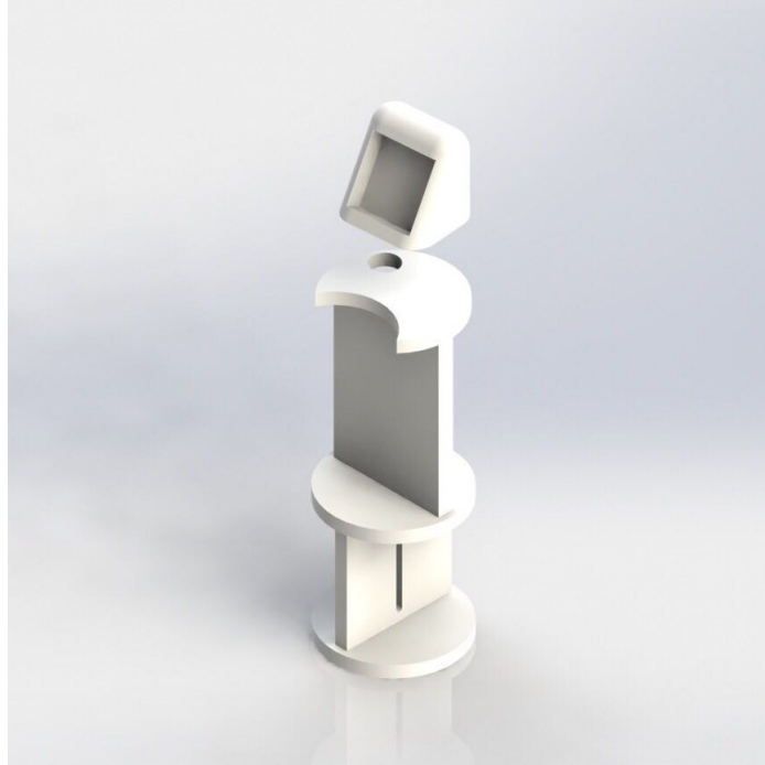
Figure 5: Avionics and Ejection Electronics Sled
