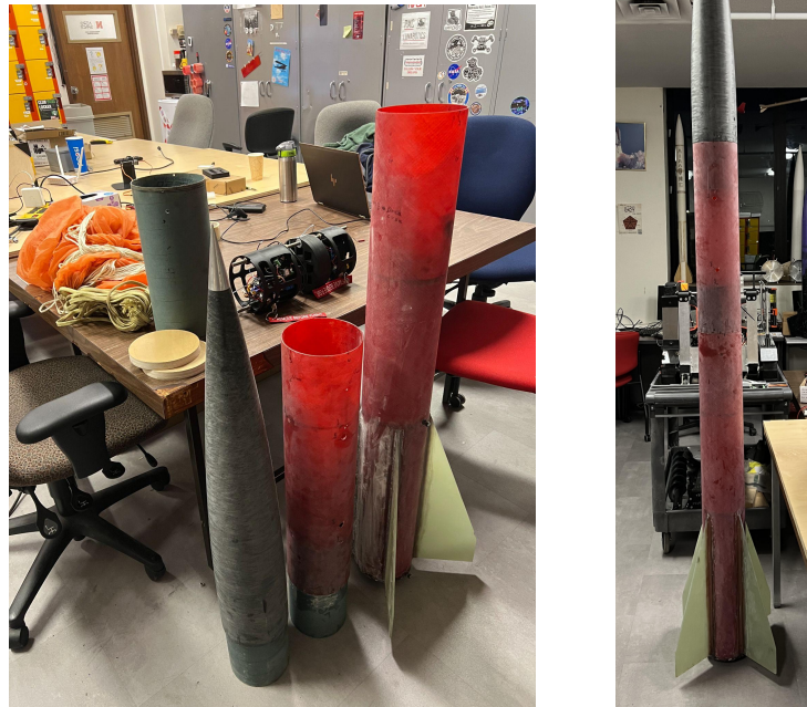
Fig. 7 Disassembled view of EVE with all components (left), EVE fully assembled (right)
