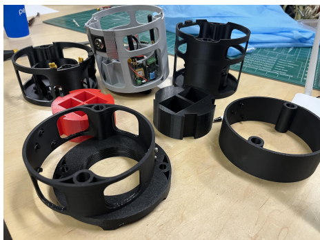
Fig. 26 Previous 3D printed design prototypes for avionics bay and payload tray
